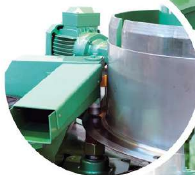
Punching of holes in the flange
