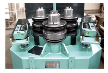
• Section bending machines: guide rolls in all their directions, pushing and pulling roll unit, mandrel and turning unit, calibration and pitch-setting devices, etc.
