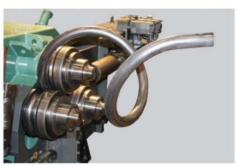
• Infeed/outfeed systems: for automatic loading and unloading of material. It is also possible to interface with industrial robots for maximum flexibility in automation.
