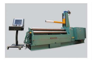
• Plate bending machines: drop end, balancing and erection of the top roll, support rolls under the lower roll, side support, top support, material infeed and outfeed systems, lifting roll, ejection device. Etc.
